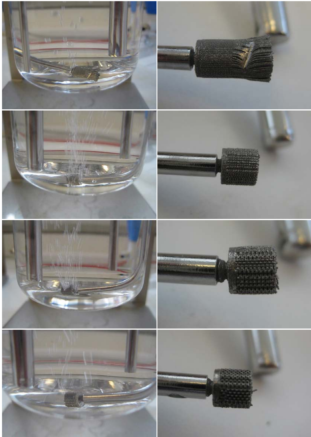
Fig. 5.27. Experimental porous spargers with a 2mm Wall and with various pore sizes: 200µm, 300µm 400µm, 500µm (from top to bottom)
