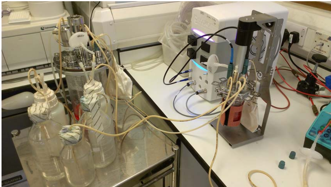
Fig. 5.16. Setup of a closed system with the MiniBioreactor in progress (right) and connected Bioreactor (3L) with BioSep (left) for the last stage of culture
