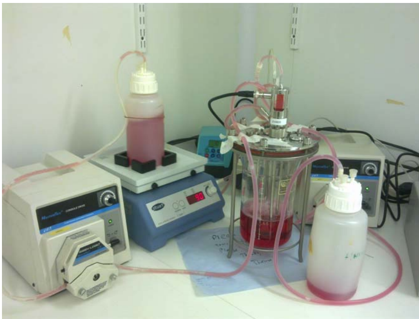
Fig. 5.3. Setup 2L bioreactor and BioSep on top of the head plate.
