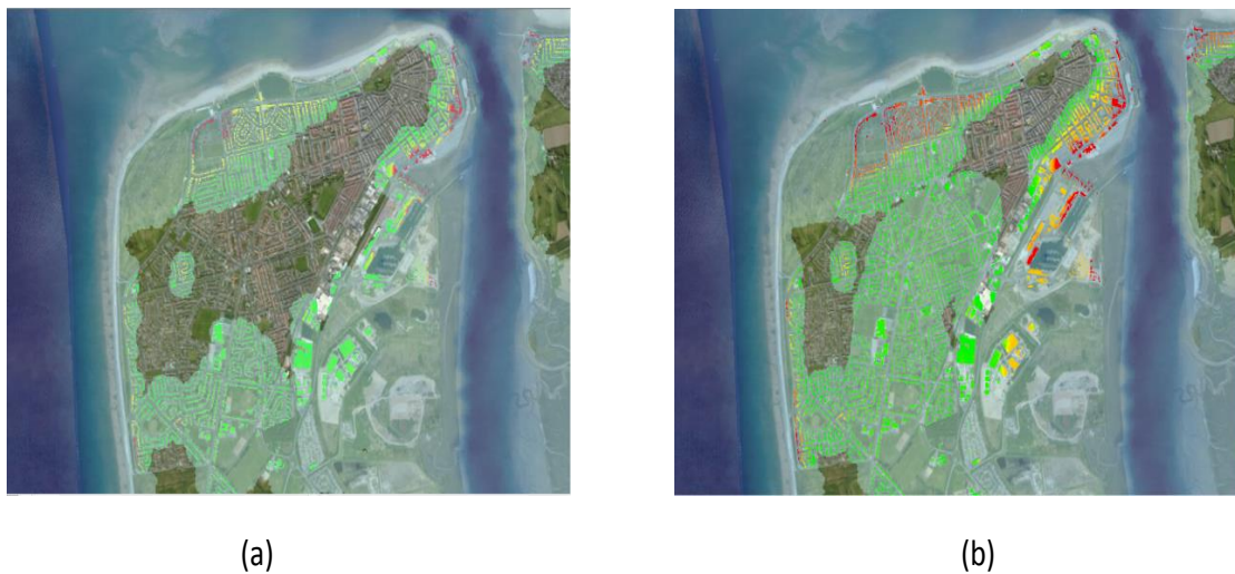
Figure 5.15 a) inundation map SLR 0cm in Fleetwood, b) inundation map SLR 49cm in Fleetwood
