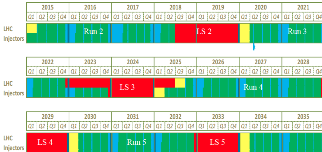
Figure 2.3: The current LHC schedule beyond LS1 as of January 2014 for both the LHC and its injectors [17]. Blocks in green refer to planned physics runs, yellow: beam commissioning, red: shutdowns and blue: technical stops.
