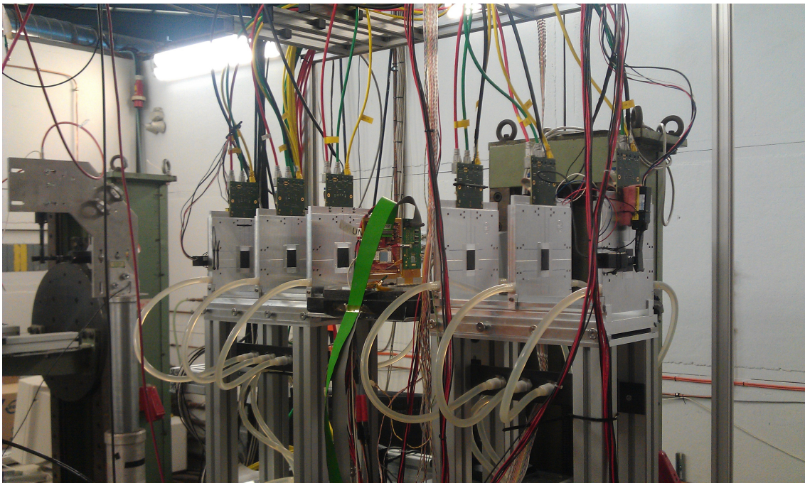
Figure 9.17: Picture of the ACONITE telescope, featuring two telescope arms with two DUT's mounted in-between. The beam direction here (DESY) travels right to left. The upstream scintillators can be seen on the far right.
