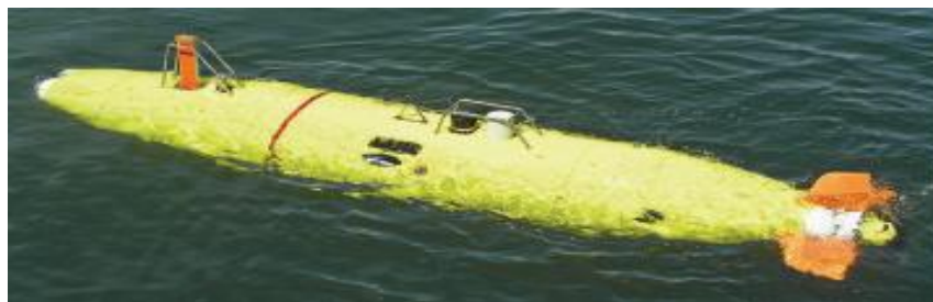
Figure 1.5. Photograph of syntactic foam autonomous underwater vehicle (Trellborg AEM).
