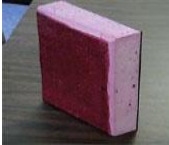
Figure 1.6. Photograph of a syntactic foam blast mitigating material (Trelleborg AEM).
