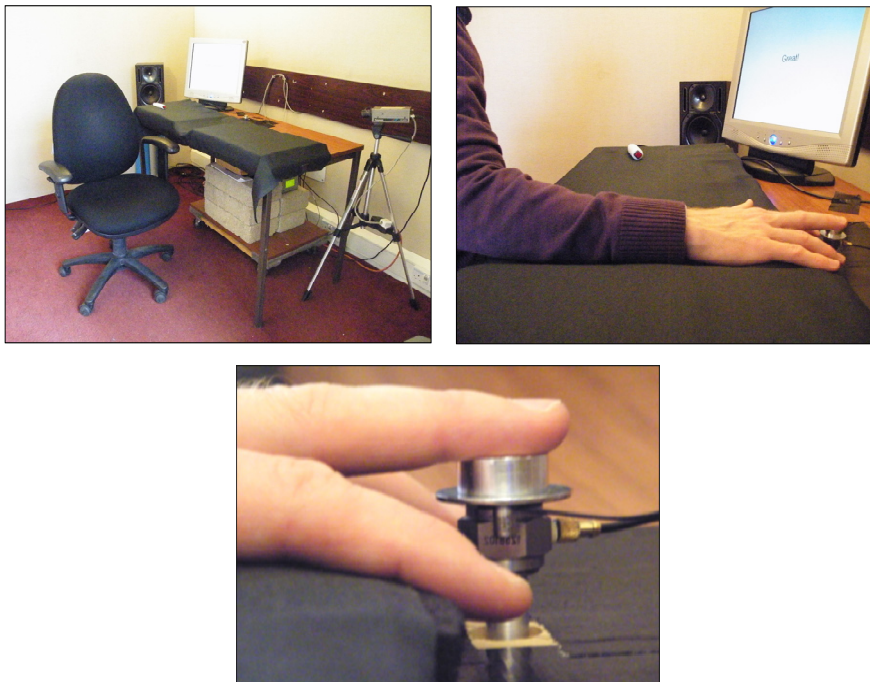
Figure 3.2 General view of audiometric booth is shown (top left) along with details of the contactor disc and a participant's fingertip being tested.
