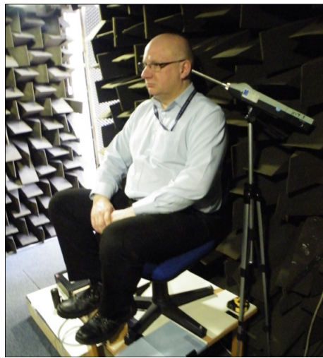
Figure 3.10 Measurement of masking noise conditions for experimental set-up.
