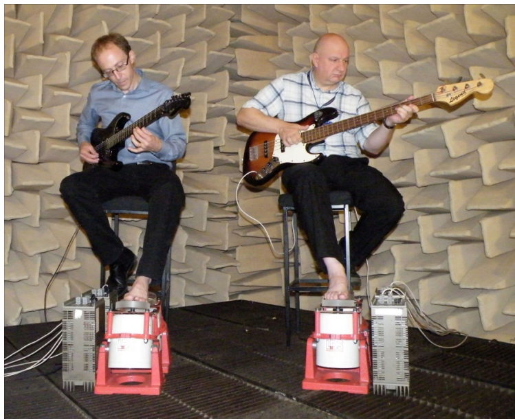
Figure 1.1 Proposed solution for two musicians, each using two vibrating footrests.
