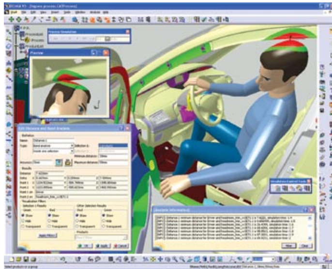
FIGURE 3.12: A head clearance analysis [102].
