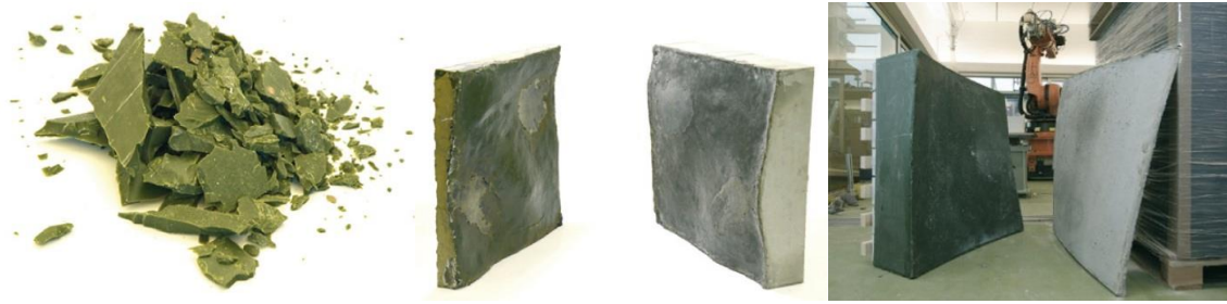
FIGURE 2.74 - 2.76. Re-usable wax; Wax negative/concrete positive; 1×1 m double curved free-form wax element, produced by a robotic process, and the concrete positive cast against it 181
