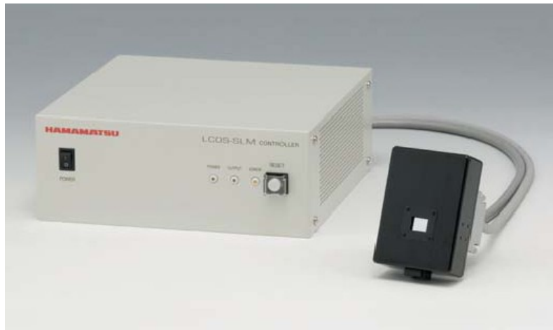
Figure 1.21: Nematic liquid-crystal Spatial Light Modulator (SLM) from Hamamatsu Photonics K.K. This SLM is made of reflective liquid-crystal pixels arranged in a two-dimensional array. The SLM is driven by a controller which provides the appropriate voltage required to drive the liquid-crystal pixels.
