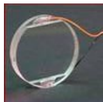
Figure 1.19: Polarization rotation device manufactured by Boulder Nonlinear Systems Inc. These devices are based on a ferroelectric liquid-crystal technology and rotate the polarization of transmitted light when an analogue voltage is applied. The polarization rotation device has a clear aperture of 25mm and its optical surfaces are coated with an anti-reflection layer for maximum transmission efficiency.
