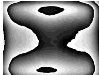
Figure 4.13: Phase correction pattern induced by a Hamamatsu X10468-02 SLM, to correct for phase distortions induced from the imperfect surface flatness of its LCOS chip. This phase correction pattern was provided by Hamamatsu Photonics K.K.
