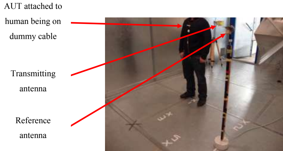
Fig. 3.3: On-body reference measurement set-up
