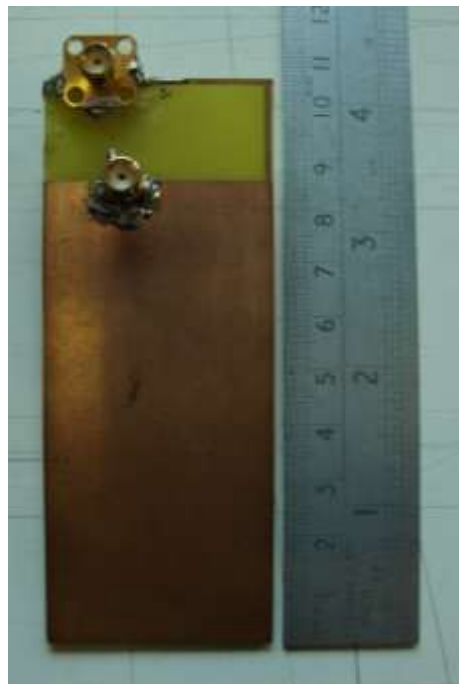
Fig. 4.3: Etching technique to provide isolation between the two feeds
