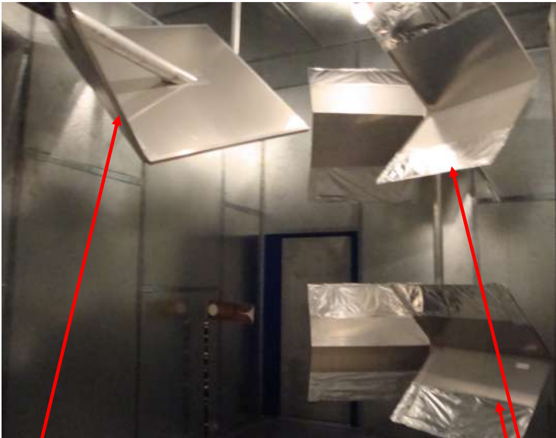
Fig. 2.9: Example of mechanical stirrer design in University of Liverpool RC
