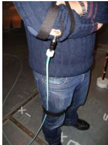
Fig. 3.19: Measurement set-up for bent elbow investigation
