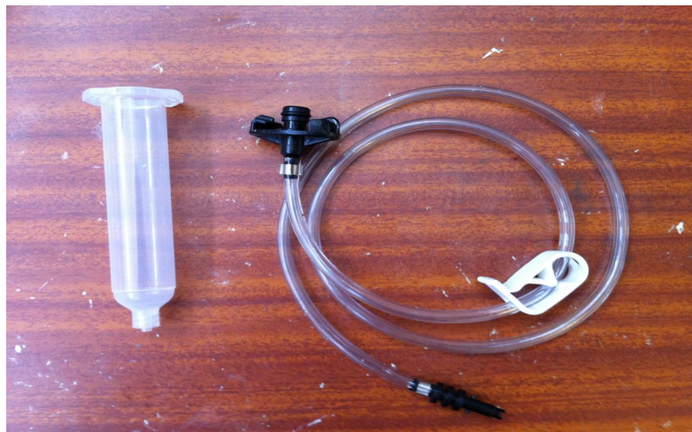
Fig 3.5. The syringe unit and gas pipe
