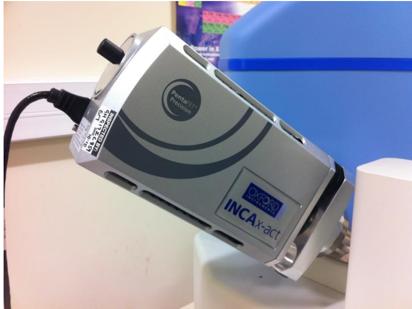
Figure 43: Oxford Instruments Inca X-act EDX analysis machine. This system was attached to the Jeol 6610 SEM.
