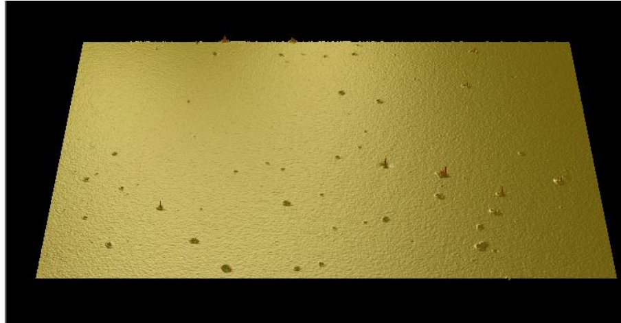
Figure 79: A white light interferometry image showing the surface of an unprocessed, uncoated glass sample. These measurements were recorded at x50 magnification.
