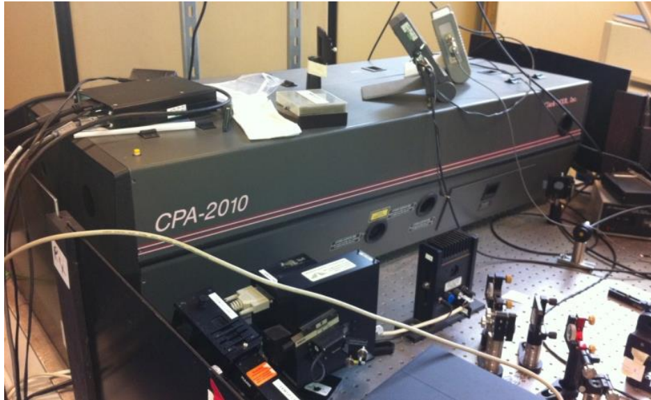
Figure 29: Clarke MXR fs laser system. This system has a split level arrangement with the seed pulses generated in the lower half before undergoing amplification using CPA in the upper half. The output wavelengths available are 387nm and 775nm the frequency is 1 kHz.
