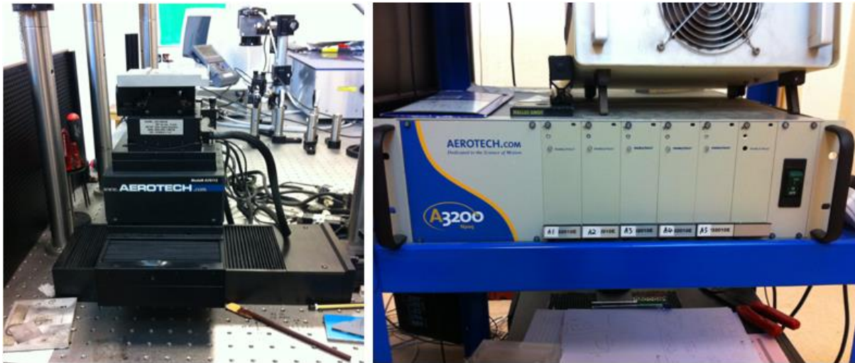
Figure 38: Aerotech stage (left) and driver unit (right). This stage was attached to the HighQ laser and provided movement in 5-axis XYZUA.
