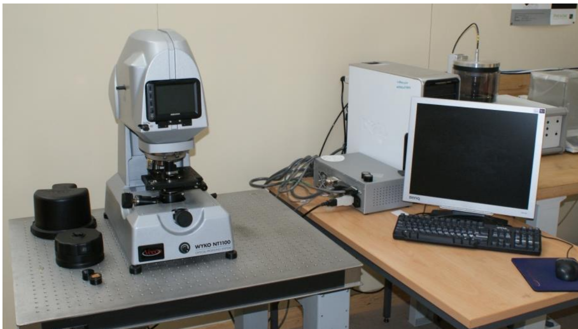
Figure 40: White light interferometry profiling system. A light source was used to illuminate the surface of a target object; interference fringes at the focal plane are used to produce an image. Measurements were initiated and analysed using the Vision software provided.
