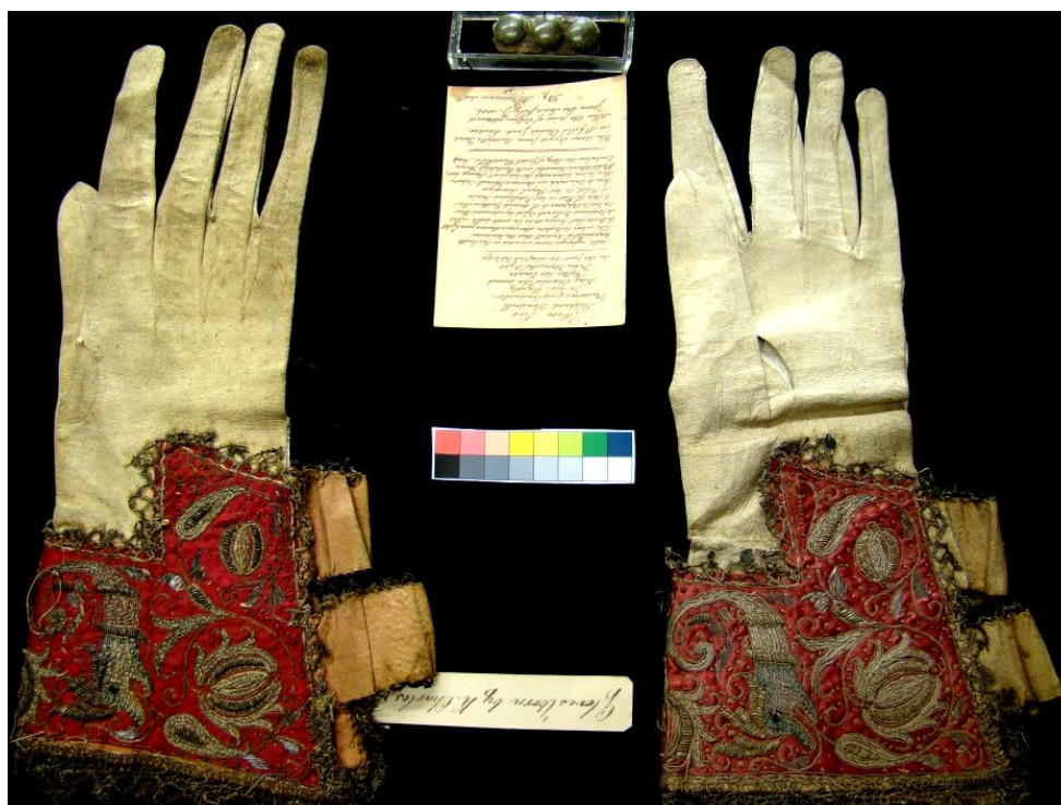
Figure 48: King Charles I gloves before laser treatment. The contamination of the white leather is clearly visible in this image. The decorated gauntlet is also shown. These images were taken from “Royal accessory under laser cleaning” by Abdelrazek et al [148] .
