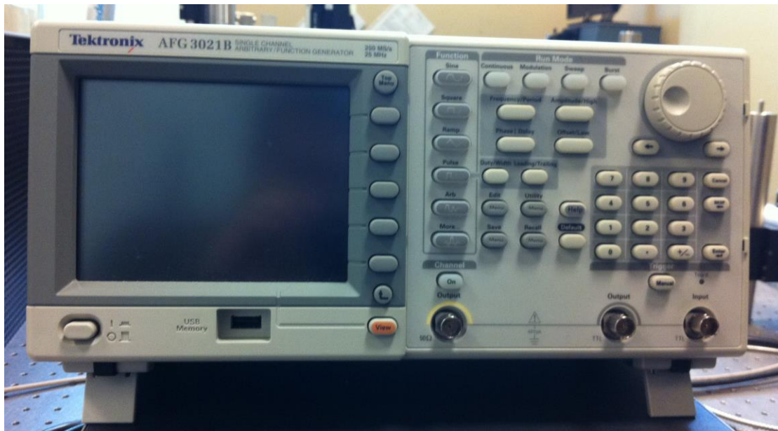
Figure 39: Tektronic function generator; using this system it was possible to gate the laser to emit a specific number of pulses. This enables the user to produce frequencies up to the maximum produced by the system.
