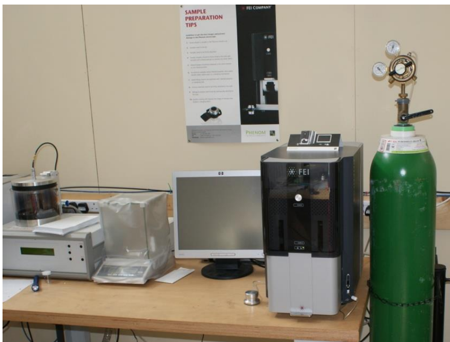
Figure 41: SEM area of LLEC. The SEM was a Phenom FEI scanning electron microscope. Samples were loaded into the base unit for optical microscopy before pumping down for SEM.
