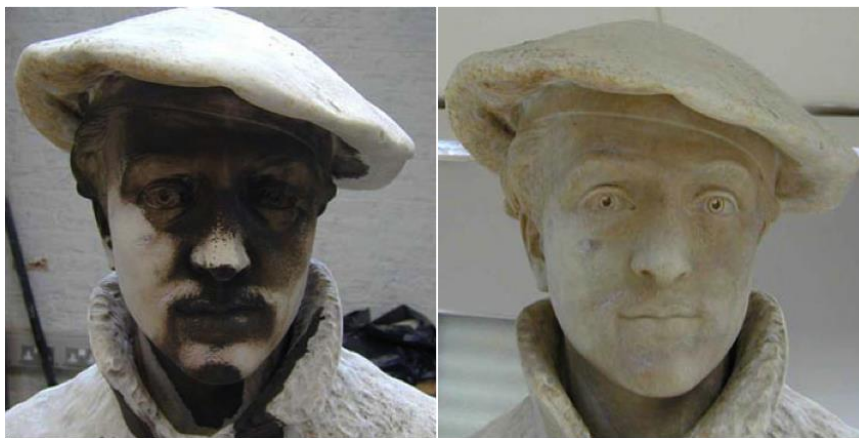
Figure 1: Laser cleaning of the statue of Linnaeus, the statue is displayed at the Palm House, Sefton Park, Liverpool. The image shows the statue before restoration (left) and after laser treatment (right). The contaminant layer consisted mainly of sulphur deposits [3] .
