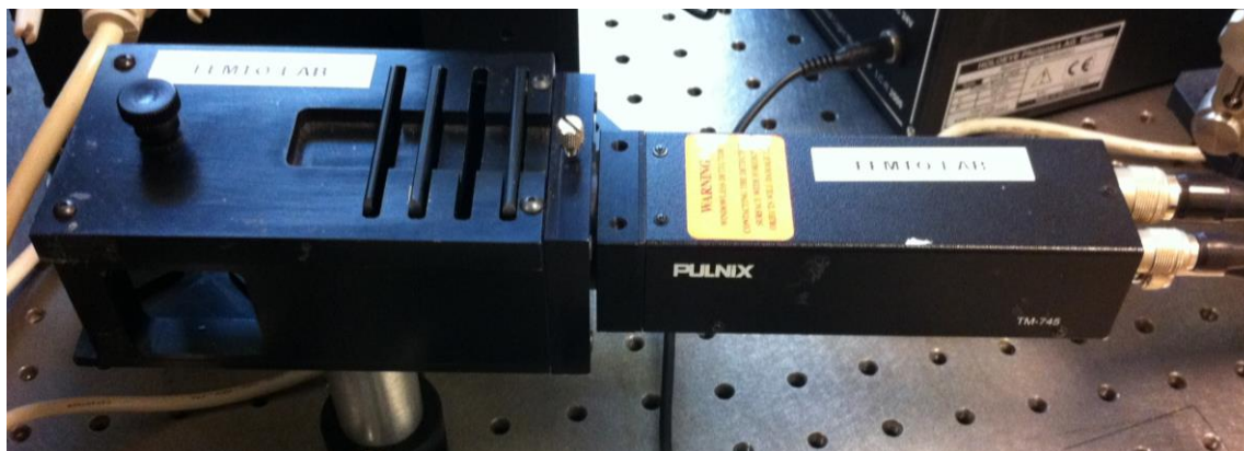
Figure 45: Spiricon profiling head. An unfocussed beam passes through a gap (left) where it is split into two components; the majority of the beam passes through but a small portion is diffracted onto the CCD (right). The recorded signal is then displayed on a PC.
