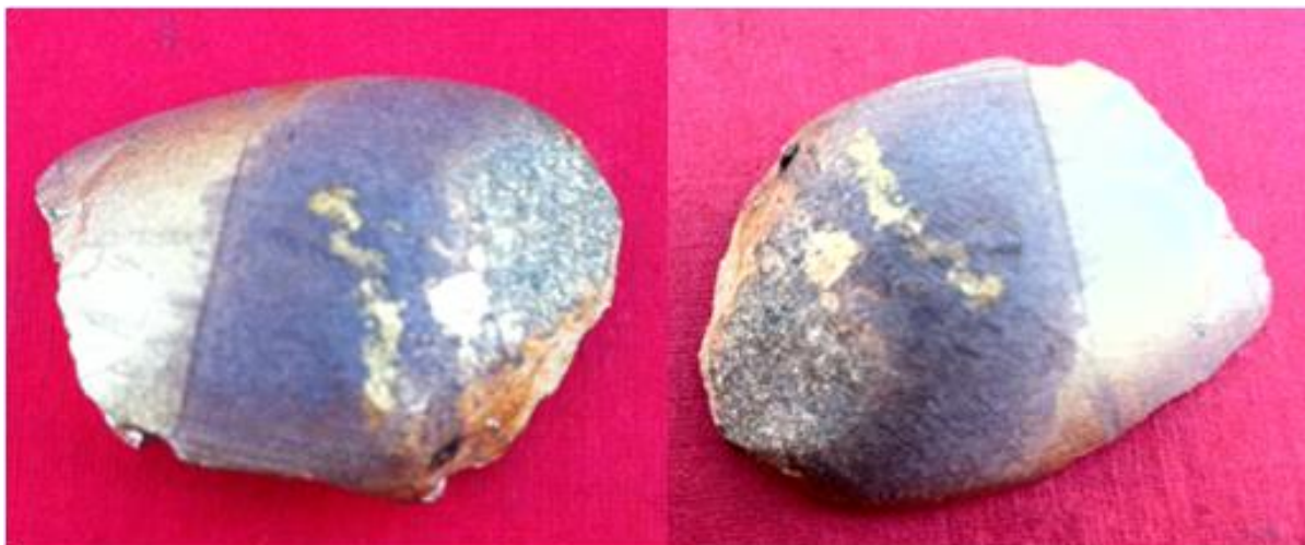
Figure 130: Using a fluence of 1.22 \text{ Jcm}^{-2} with a traverse speed of 500 \text{ mm/s} and a maximum 20 scans, the gilded frame section was irradiated to test the use of laser treatment on real conservation items. The bronze gilding on the surface was removed revealing the wood base and some gold leaf, which had previously been covered hidden due to the addition of the second gilded layer.
