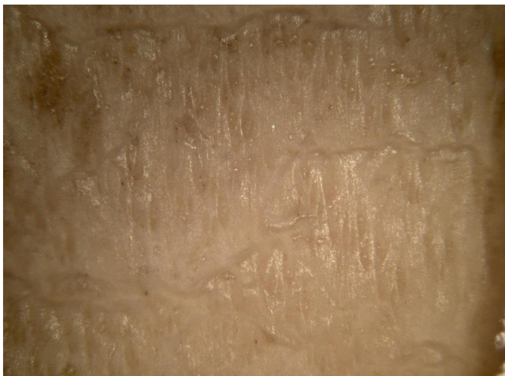
Figure 103: An image showing a section of leather restored using a fluence of 4.10 \text{ Jcm}^{-2} when viewed at x80 magnification. No surface damage was observed, however some small contaminant deposits remain on the surface.
