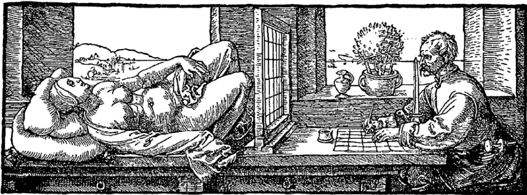
Figure 4.1: Illustration of the draftsman's net, a device to aid perspective drawing by Albrecht Dürer. The grid cuts through the field of vision splitting it into a grid which is then transferred to paper. Image credit: Dürer ([1525] 2011).
