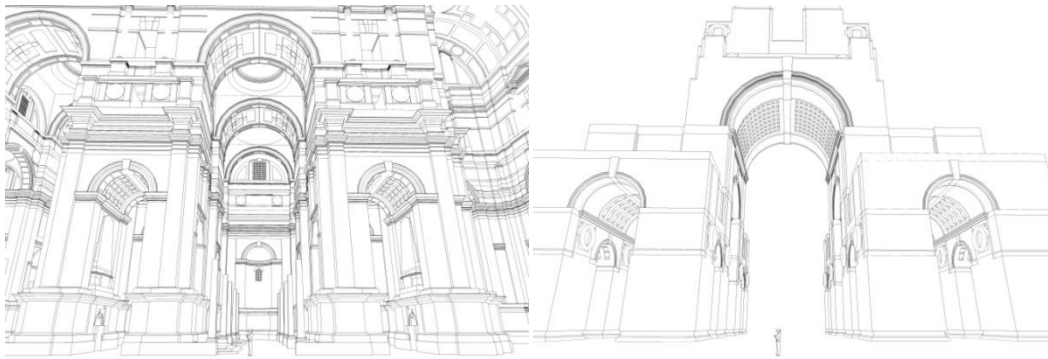
Figure 7.27: Digital line drawing of the cathedral (left) taken from the same position as Thiepval (right) looking through the 32 foot (9.75 metre) wide arch.
