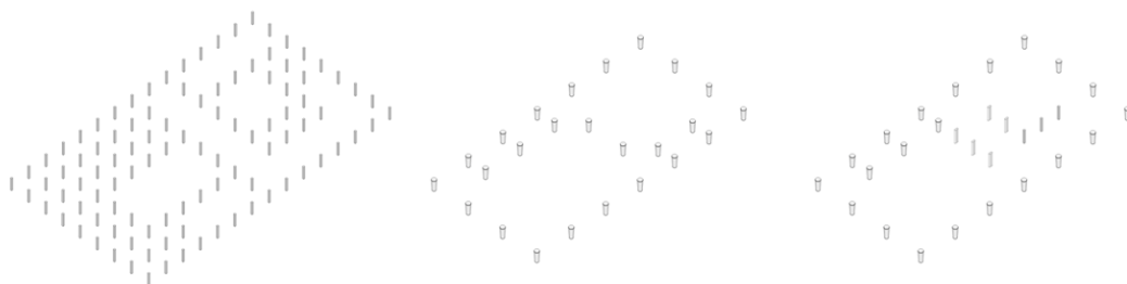
Figure 5.23: The ground floor columns developed initially by following the pattern of the above floors (left). Next they became larger and circular (centre). Finally a combination of the two with additional rounded rectangular columns was used (right).
