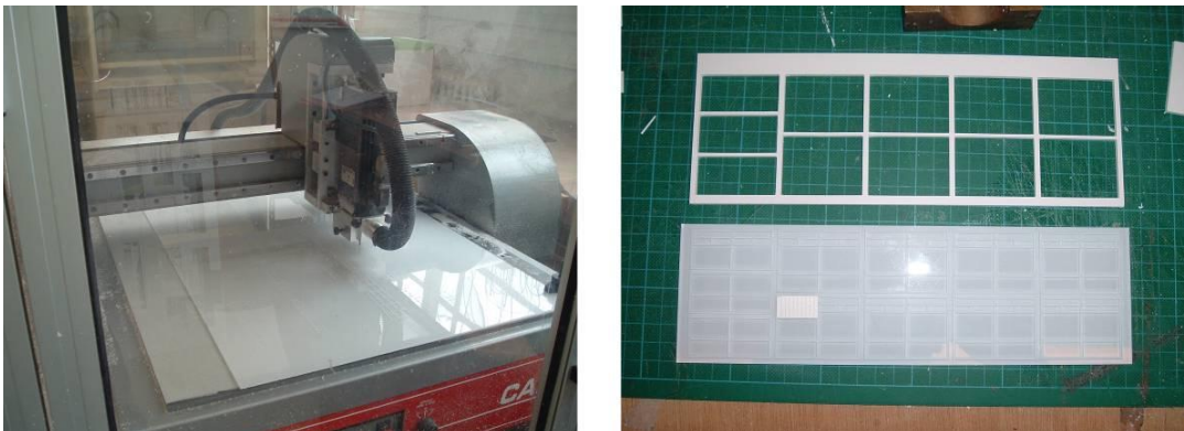
Figure 5.10: Above left: the router arm cutting various sections of the transparent acrylic to form the glazed elements of the design. Above right: the 3mm foamex sits above the acrylic once it has been finished by hand.
