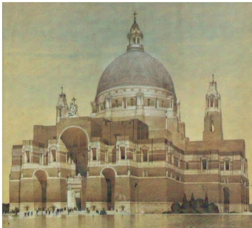
Figure 7.1: Cecil Farey perspective of Lutyens’ early design for the Liverpool Metropolitan Cathedral in September 1930. The buttressing around the dome is a lot less substantial than the later scheme. Image credit: Farey (1930).
