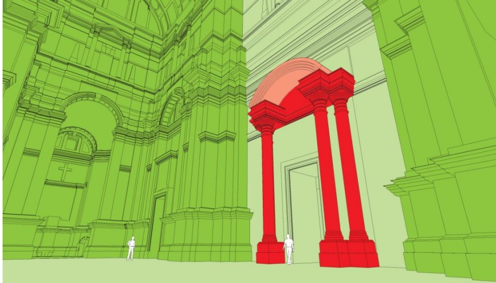
Figure 7.15: Snapshot of the narthex of the digital model indicating confidence levels in the source data based on Kensek et al (2002). Bright green represents greater confidence and bright red represents less confidence. Darker hues represent greater confidence than lighter hues giving a four tier system of confidence.
