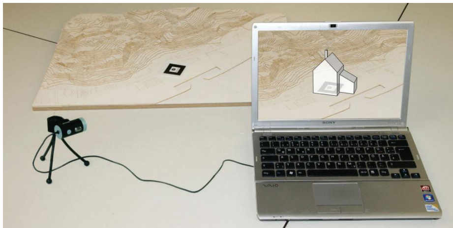
Figure 4.11: Classic set up of augmented reality. Image credit: Koch et al. (2011, p.844).
