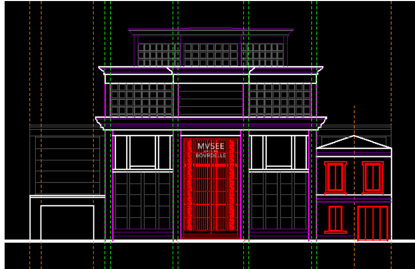
Figure 6.11: Digitally traced drawing of the front elevation. Only five square infill panels fit height wise on the drawing whereas seven are indicated on the archive perspective.
