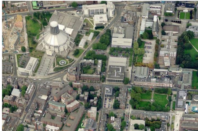
Figure 4.4: Bing maps use ortho-rectified images to provide an axonometric projection or bird's eye view. This allows for scrolling in any direction. Image credit: Bing maps (2010).
