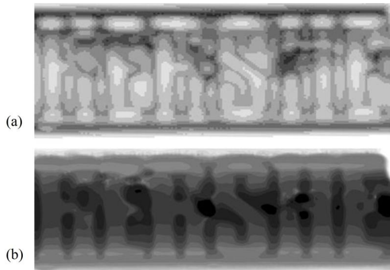
Figure. 2.14 THz transmission images of a chocolate bar obtained by using (a) peak-to-peak amplitude of the transmitted time-domain pulse and (b) variation in transit time of the THz pulse through the sample. Figure adapted from [77].
