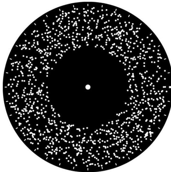
Figure. 5.16 Schematic diagram of new generation spinning disk which is made of a 20.0 mm \times 20.0 mm steel plate. The diameter of each holes drilled on the plate is 2.0 mm.
