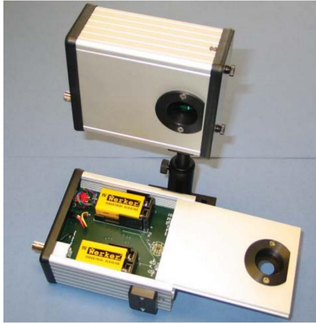
Figure. 2.6 A photo of pyroelectric detector (SPH-49, Spectrum Detector Inc. USA). NEP=3\times 10^{-9} W/Hz^{1/2} .
