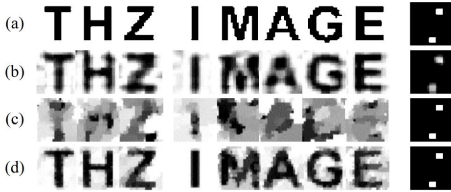
Figure. 4.2 Simulated results demonstrating the universality of the proposed mask. (a) Original image and reconstructed images using (b) 40 optimized masks, (c) 40 random masks, and (d) 120 random masks [5].
