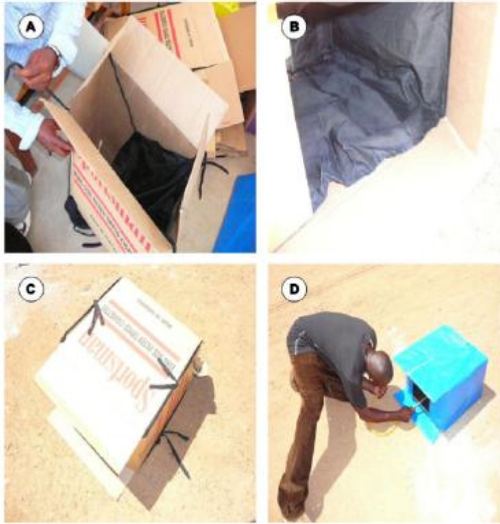
Figure 4.3.1: Photographs of resting boxes. A and B illustrate how the boxes are made, C demonstrates how to install them and D demonstrates how to recover resting mosquitoes (Sikulu et al. 2009)
