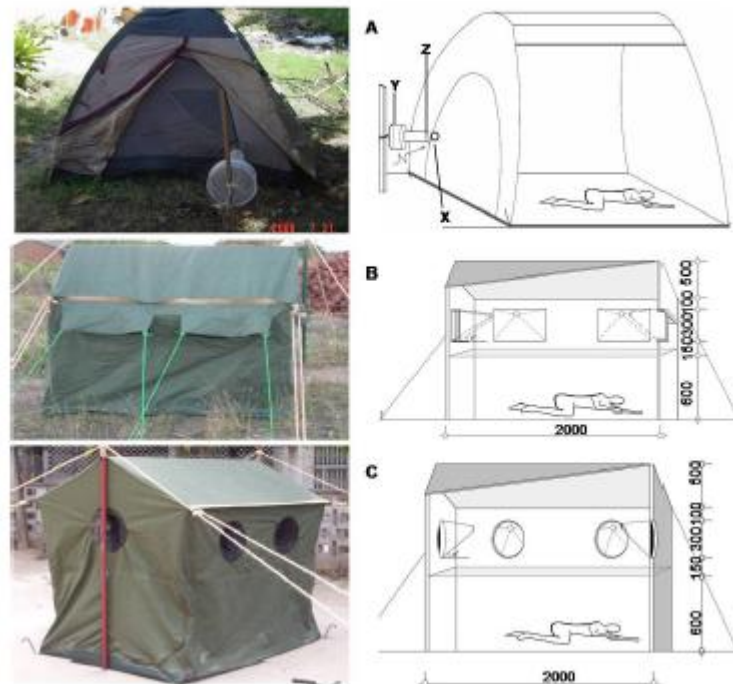
Figure 3.3.1: Furvella trap (A), Ifakara A tent trap (B), Ifakara B tent trap (C), with section drawing of each. The human occupant is protected from mosquito bites by a netting panel within the Ifakara A and B designs. For the Furvella trap, mosquitoes approach the small opening in the tent zipper (X) where they are drawn into the collection bag (Y) when they pass the CDC light trap entrance (Z), while in the Ifakara designs they enter through a funnel shaped entrances tilted upward. All dimensions in mm.
