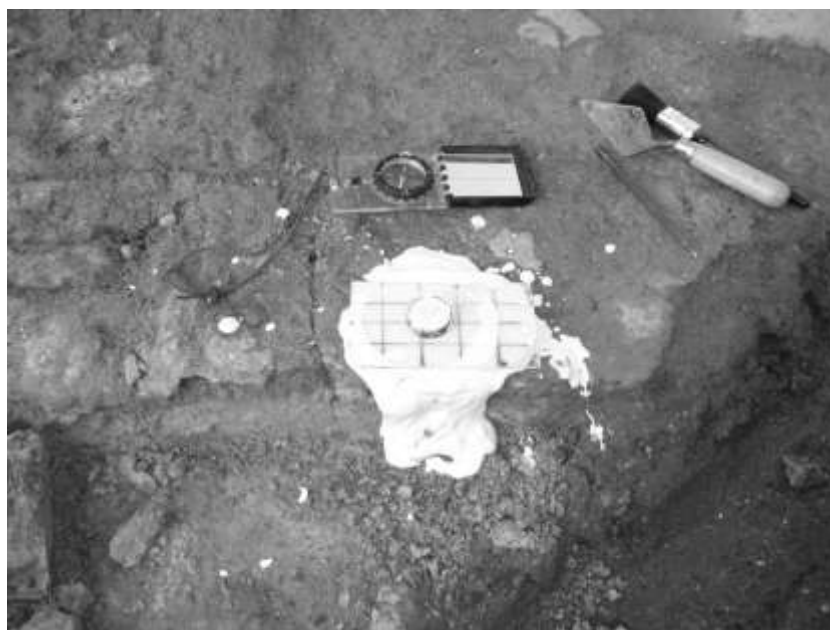
Figure 14.1 Photograph of sampling procedure, showing plaster with bubble level.
