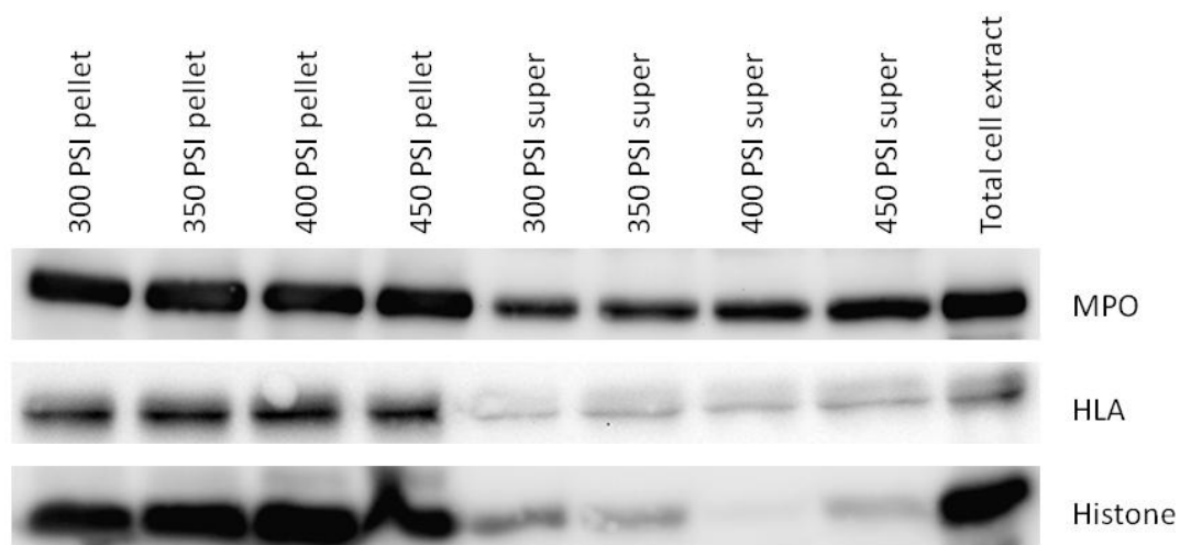
Fig.36. The amount of MPO in the supernatant progressively increases with increasing bomb pressure. The lower the bomb pressure the greater the number of unlysed cells (larger pellet). Therefore, a bomb pressure of 350Psi was chosen to maximise the number of cells lysed but minimise the granule disruption.
