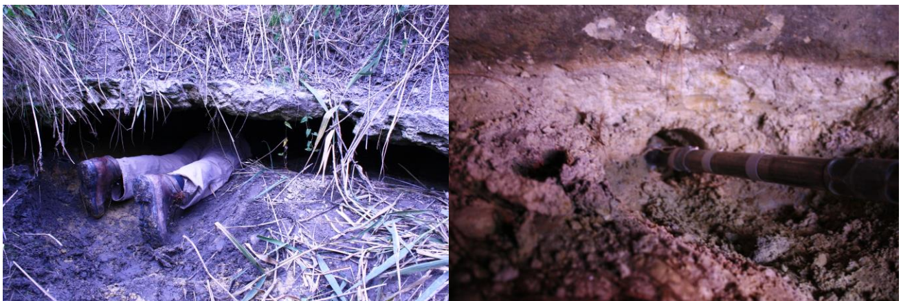
Fig. 2 Sampling at the exposure beneath the carbonate bench by using steel cylinders
