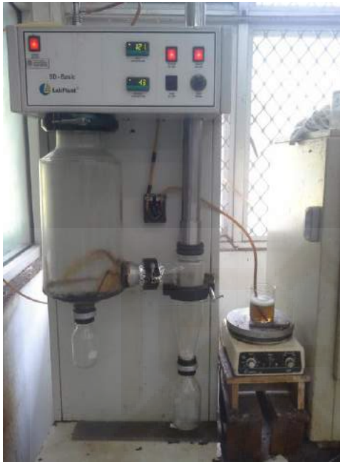
(f) Proses Spray drying
