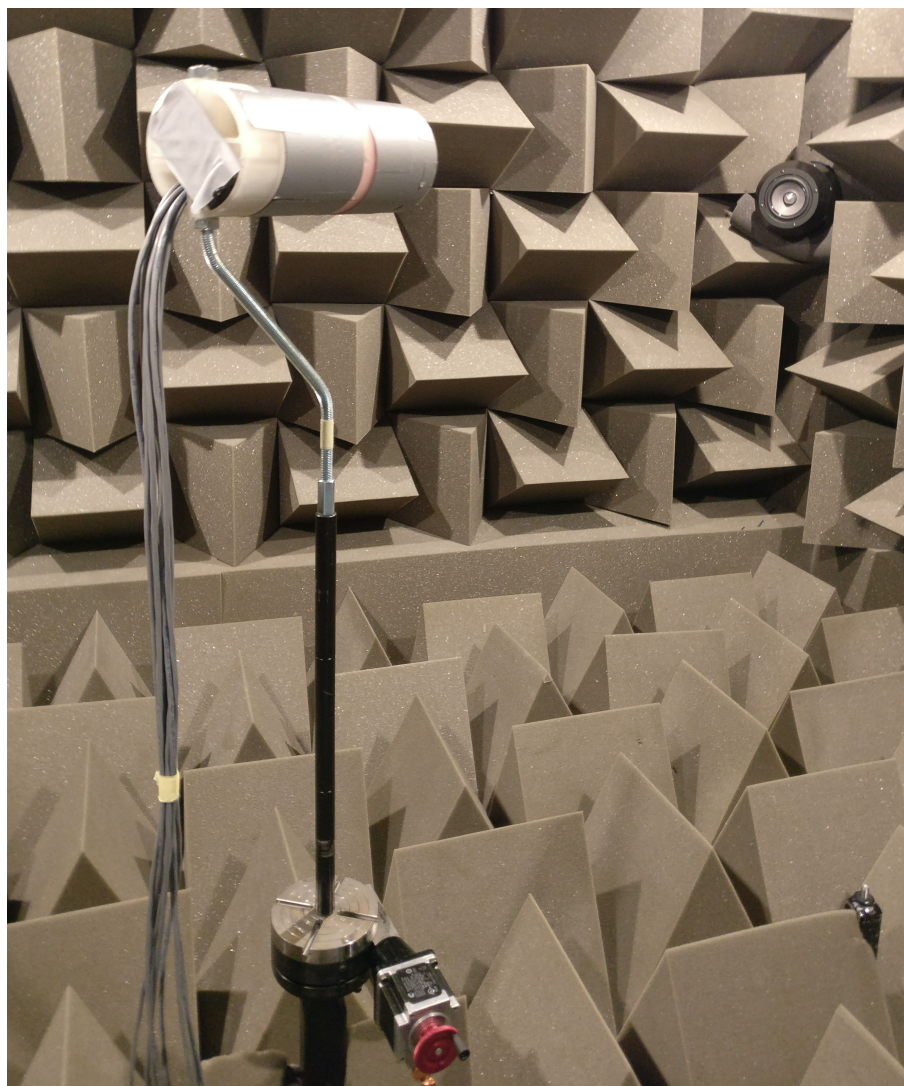
Figure 16: A photo of the baffled circular array in the measurement system when measuring the responses at different elevation angles.
