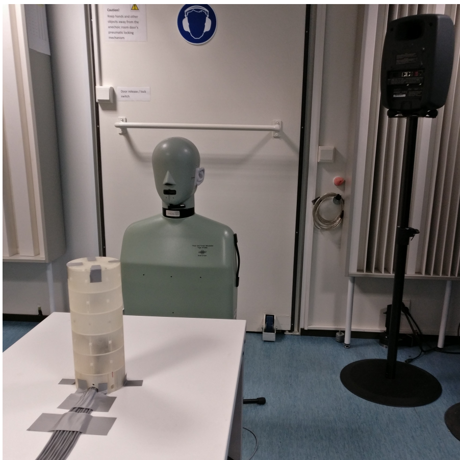
Figure 18: A photo showing part of the measurement setup: the array, the Head and Torso Simulator and a loudspeaker used to generate the noise field.
