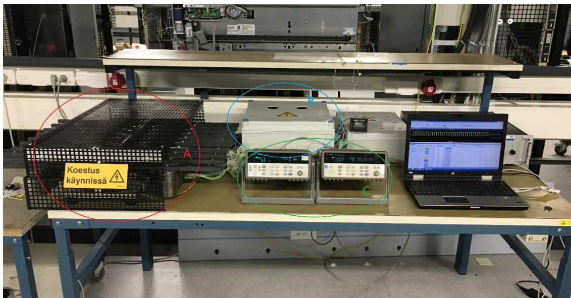
Figure 27: Test setup. A) The mechanical test frame with a contact protection. B) PCBs in a protection BOX. C) Measuring devices.
