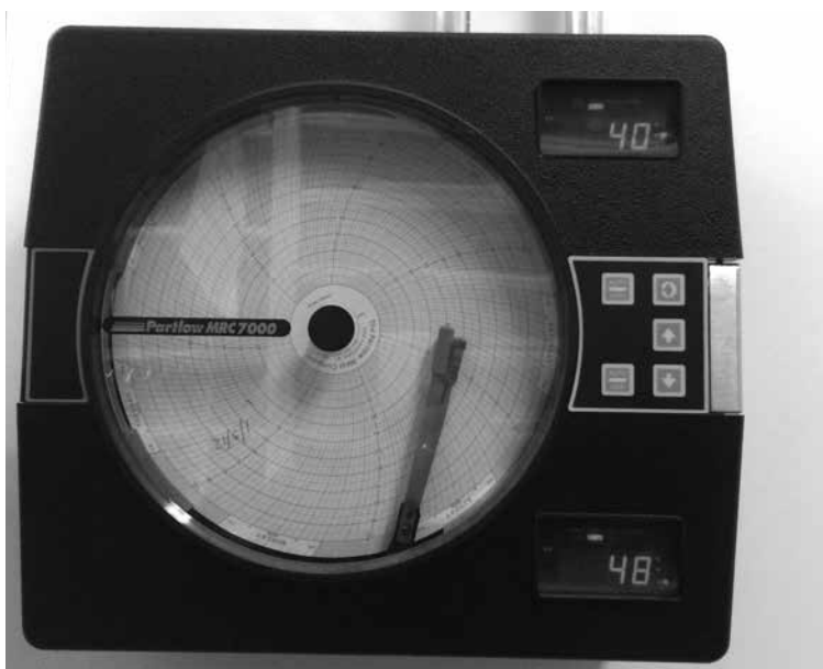
Fig. 1.6. A Circular Chart Recorder at the Cooper Hewitt's storage facility. It is microprocessor-based and capable of measuring, displaying, recording, and controlling indoor environment conditions. Photograph by Samir Bhowmik, available under a CC BY 4.0 license.
