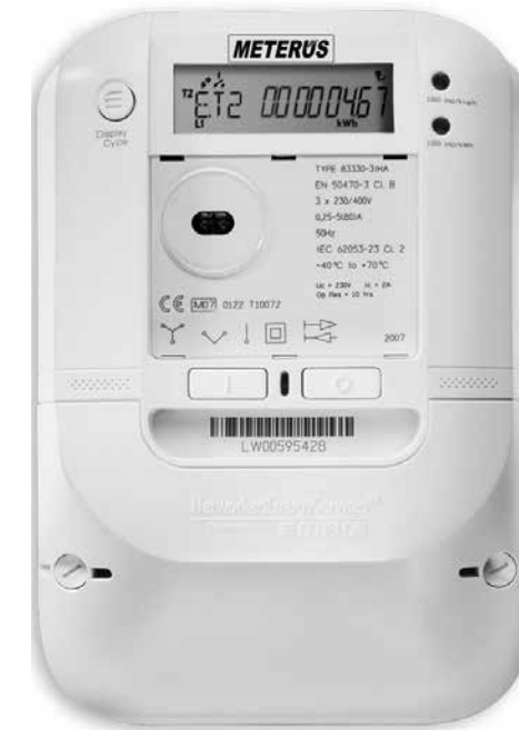
Fig. 4.7. A typical smart meter, used by EVB Energie AG. It uses two way communication to reduce load, and connect/reconnect remotely, and also interfaces for gas and water supply. Photograph by EVB Energie, distributed under a CC BY-SA 3.0 license.
