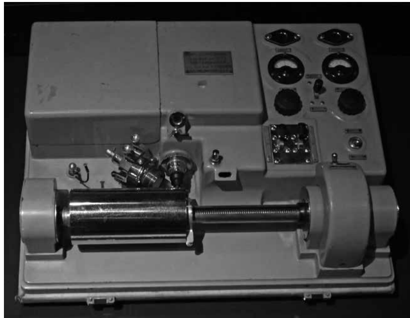
Fig. 5.5. The Belinograph BEP-2V telephotograph by Edouard Belin. Photograph by Sandstein, distributed under a CC BY-SA 3.0 license.
