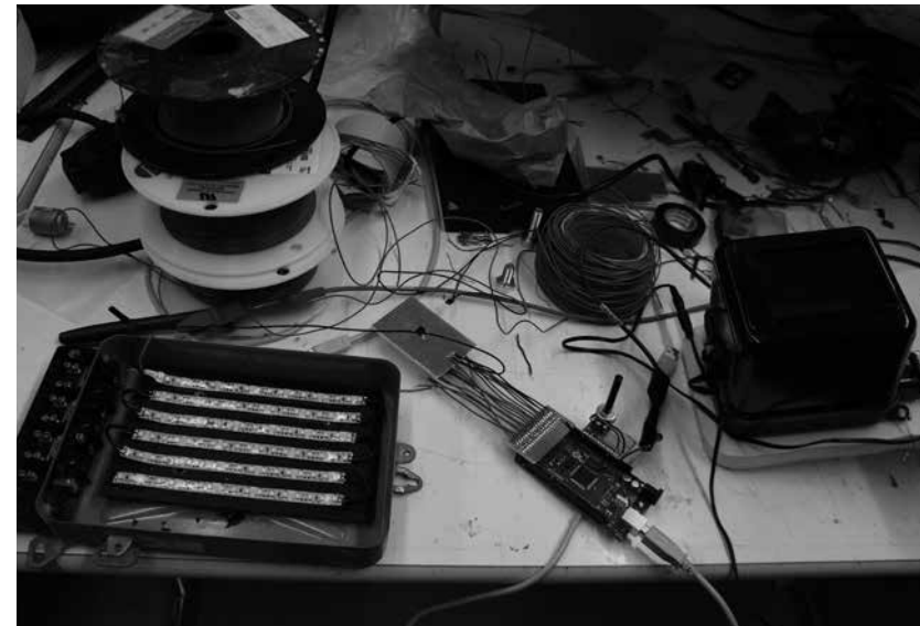
Fig. 4.25. The Arduino connected to the LED strips.
