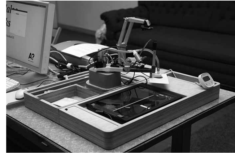
Fig. 5.13. Old scanner embedded into a ‘new’ scanning system.
