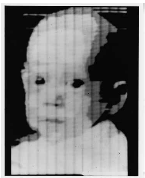
Fig. 5.7. The first scanned image, outcome of the first drum scanner to be used with a computer built in 1957 at the US National Bureau of Standards. The image was a 5 cm square (black and white, 176 pixels) of Russell A. Kirsch's three month old son. Photo courtesy of National Institute of Standards and Technology.
