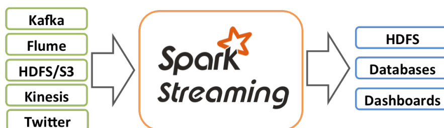
Figure 18: Spark Streaming Architecture (Source: [6])
