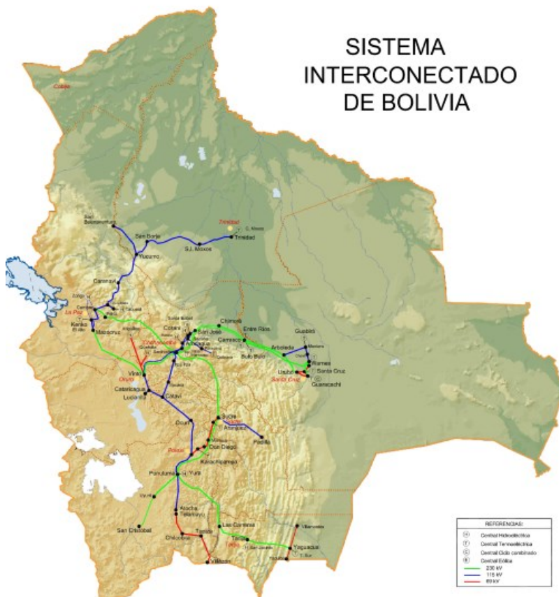
Figure 11 National Electricity Grid of Bolivia [31]
