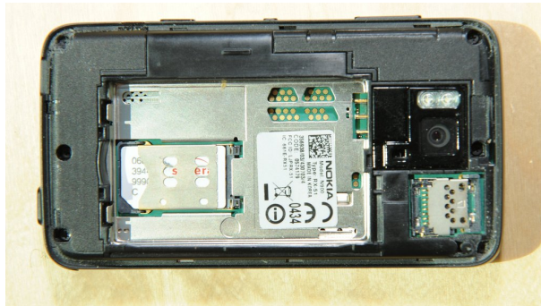
(b) Nokia N900 backside where the debug pins are visible. The TX pin for the serial port is on the right bottom pad's left upper corner. The bottom pad's left lower corner is the RX pin.
