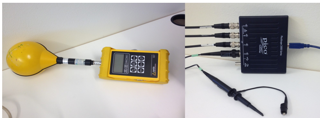
Figure 4.2: a) Narda's ELT-400 Exposure Level Tester for magnetic fields and b) PicoScope 2406b from Picotechnology
