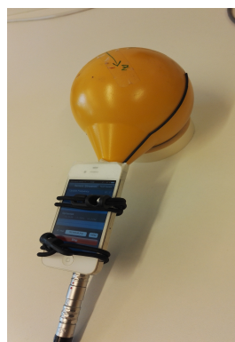
Figure 4.10: The smart phone iPhone 4S collects data about the orientation of the magnetic field probe.
