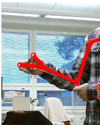
Figure 5.4: The small hand-made probe tracked with Kinect's skeletal tracking.
