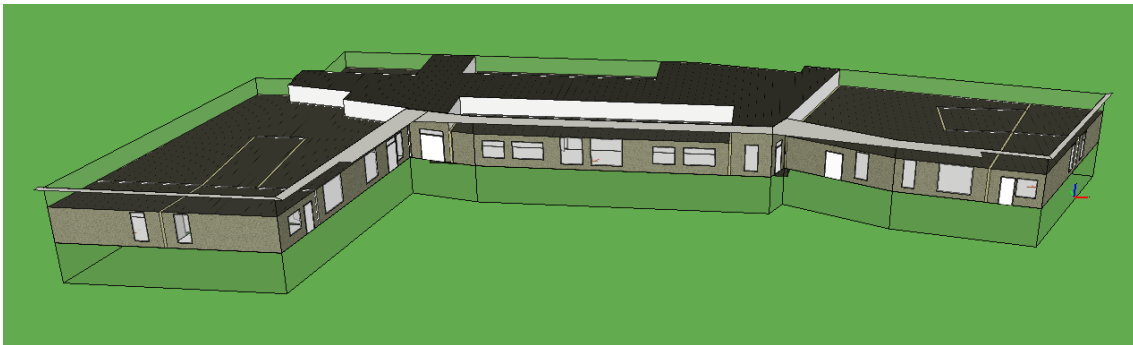
Figure 13. IDA-ICE model showing the building envelope of Luhtaa day-care centre, without the existing solar panels.
