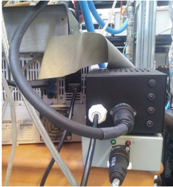
Figure 5.18 Optocoupler and power supply of the electronic control system for solenoid valves.
