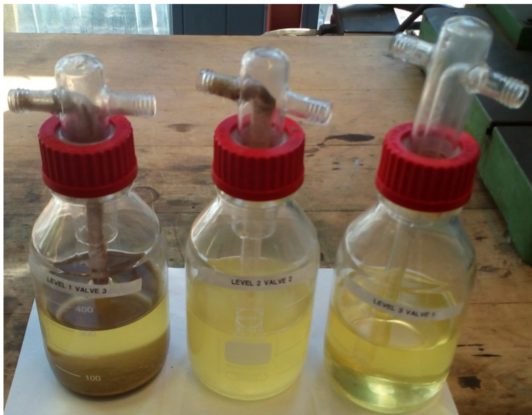
Figure 7.7 Tar trap (oil scrubbers) with retained substances after one combustion test in the reactor.
