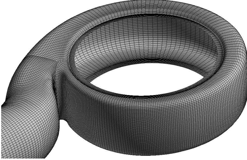
Fig. 2: Surface grid of the volute.
