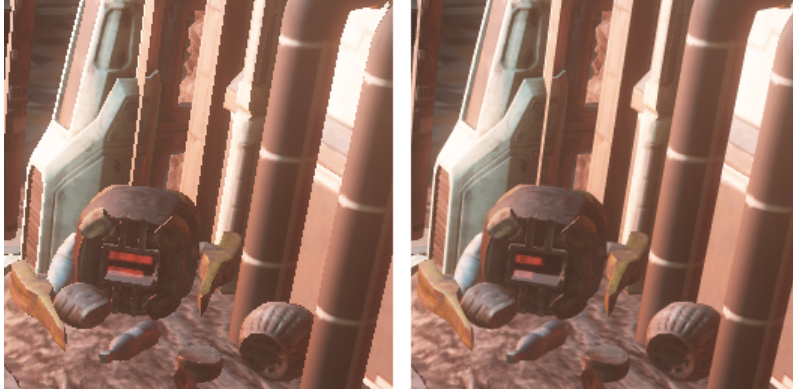
Figure 1.1: Picture on the left show jagged geometry edges. On the right jaggies do not exist due to anti-aliasing. Both images have been rendered with the same resolution.
