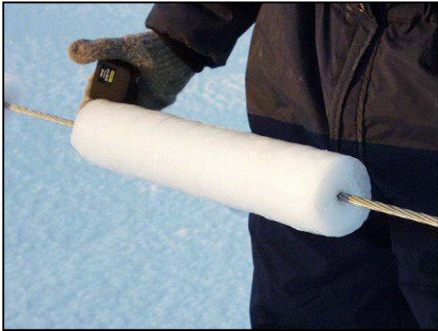
Figure 4.9 Ice on Conductor [28]
