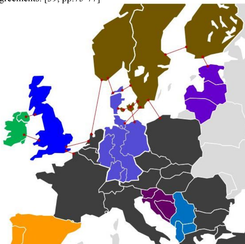
Figure 9: The five synchronous areas in Europe and their division into smaller operational areas. [39, p.42]
