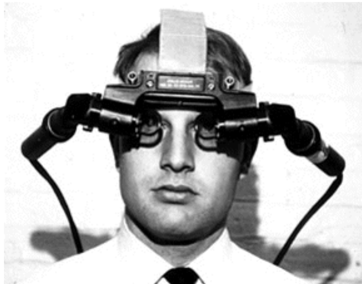
Figure 1: Optics of the first head-mounted display in 1968 [11].
