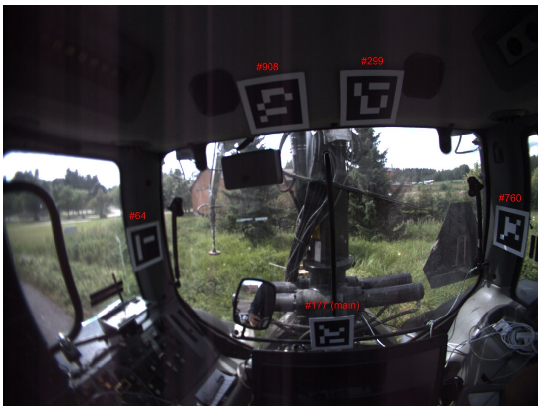
Figure 18: The view inside the tractor cabin. IDs of the visible markers are marked in red.
