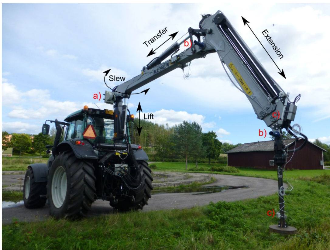
Figure 12: Tractor and forestry crane used in this work [83]: a) laser scanner, b) markers, c) IMUs.
