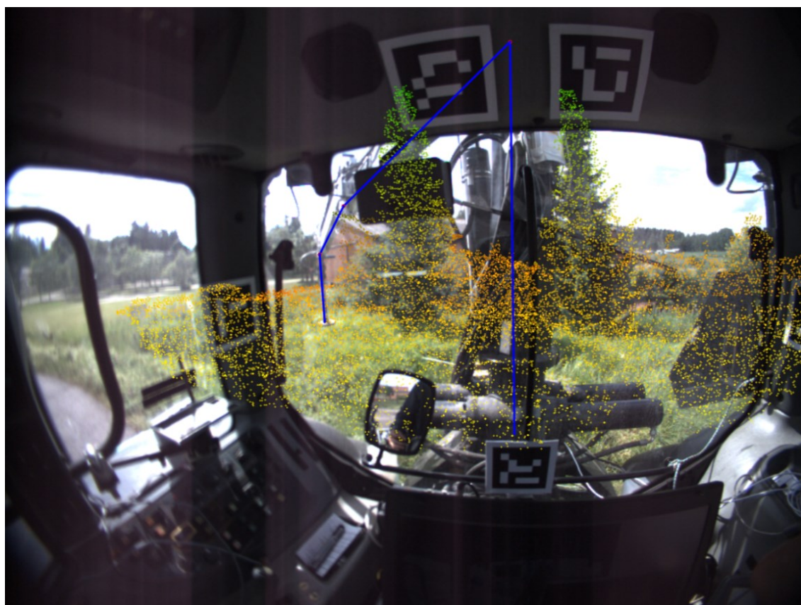
Figure 19: An augmented image from the video. The crane and the tool is shown in blue along with the point cloud data from the lidar.
