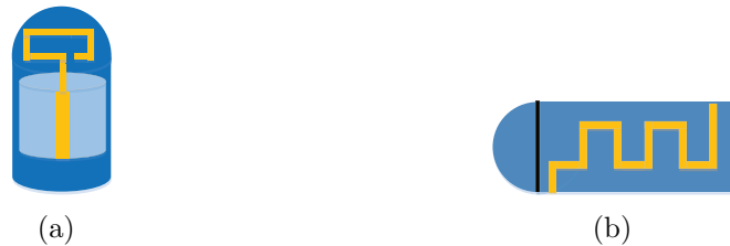
Fig. 11: Antenna types for a capsule transmitter: (a) embedded antenna inside a capsule module; (b) conformal antenna around the outer surface of a capsule module.
