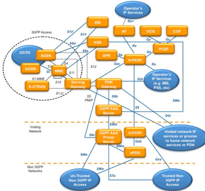
Figure 4.3: Diameter Interfaces in LTE [23]
