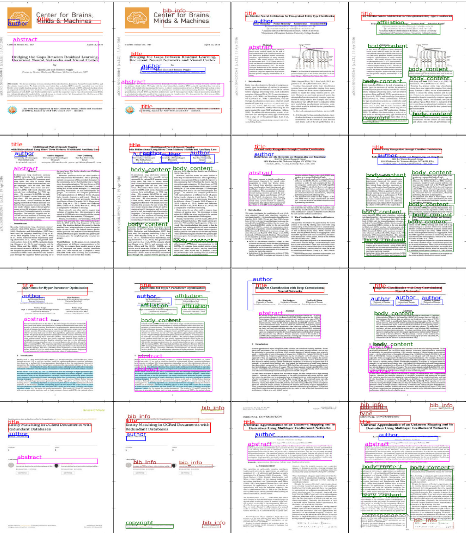
Figure 17: Comparing of the output of VGG-16 with a multi-256-softmax and Faster R-CNN. The first and third column are the results from VGG-16 and the second and fourth column are Faster R-CNN predictions. The Faster R-CNN predictions only show the prediction with the highest confidence for a given region.
