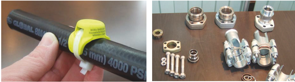
Smart Care Hose Management System RFID attached to the hose, and examples of flange connections.
