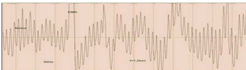
Fig. 11:50 Hz noise in the signal.
