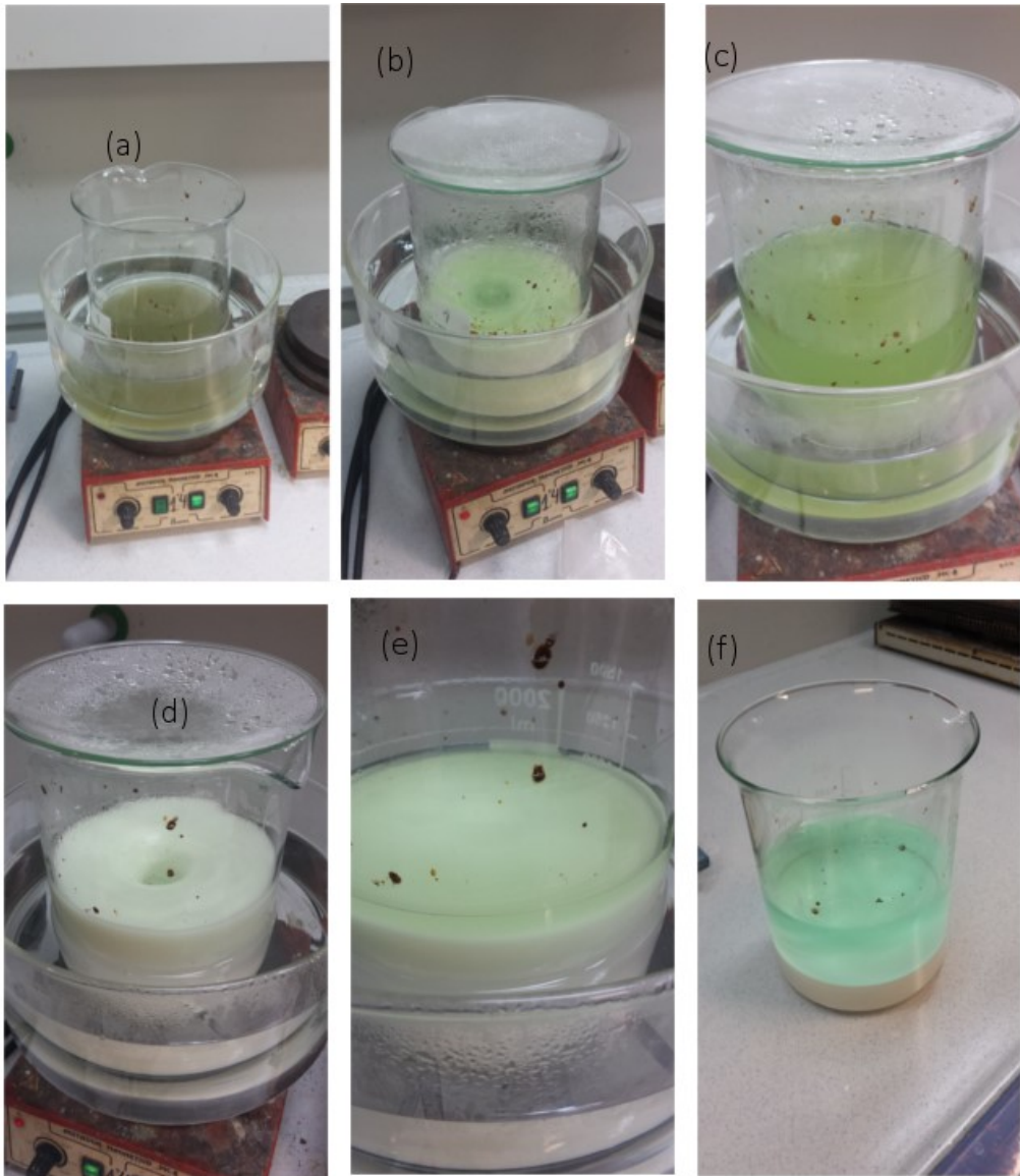
Figure 22. The scorodite precipitation procedure: (a) set up after oxidation, (b) precipitate forms upon temperature rise, (c) after dissolving with acid the precipitate formed, (d) after gypsum seed addition, (e) the green colour is noticeably fading away mid-precipitation, (f) the solution after 5 hours.
