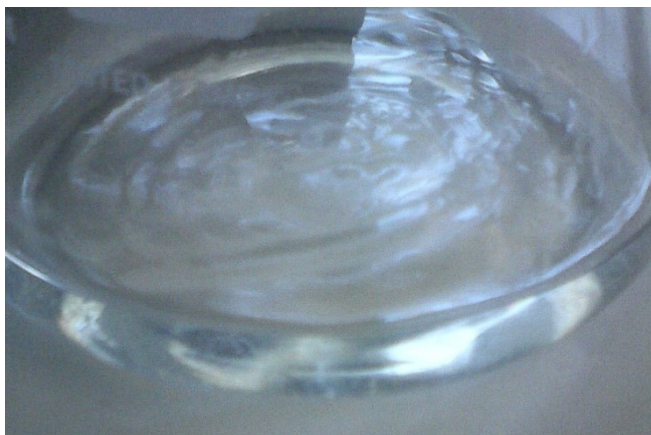
Figure 18. The filtrate is a clear solution, indicating that the process has successfully removed most of the dissolved metals from the original solution (of brown/red colour after oxidation).
