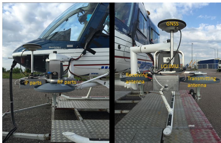
Figure 24: TomoRadar installation on helicopter
