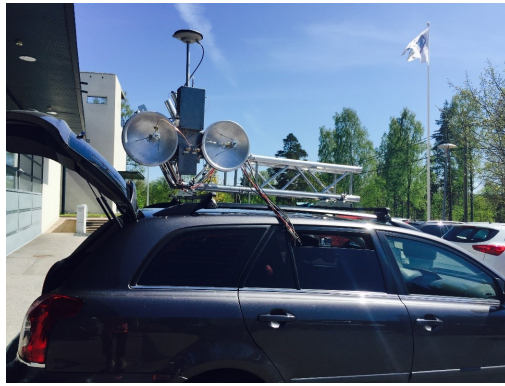
Figure 13: TomoRadar system fixed on car
