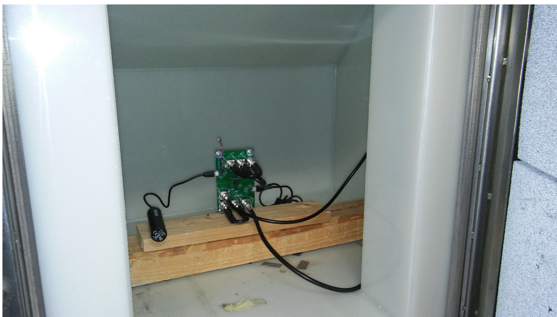
Figure 46: PCB placement in the chamber at upward position.
