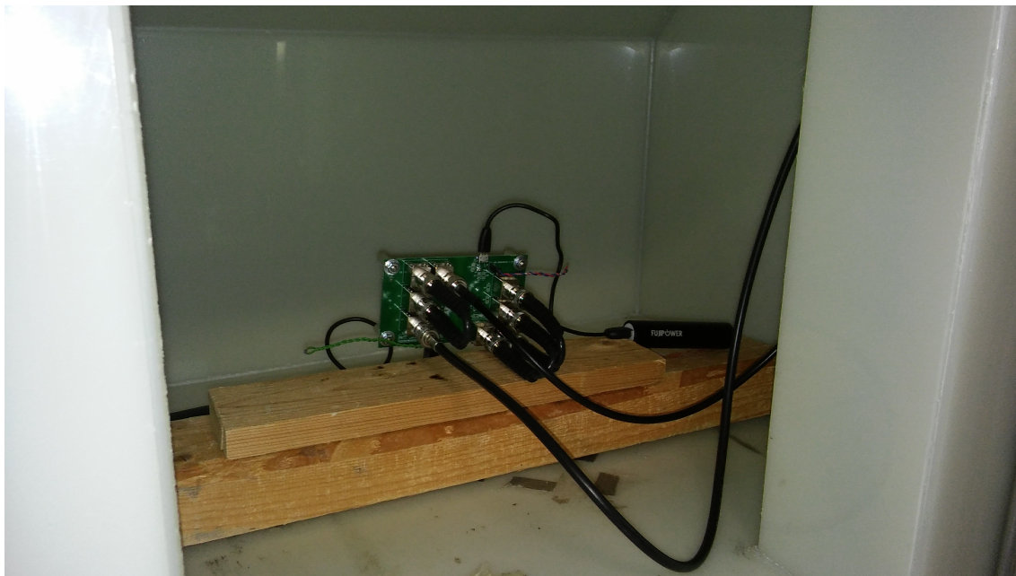
Figure 45: PCB placement in the chamber at sideways position.
