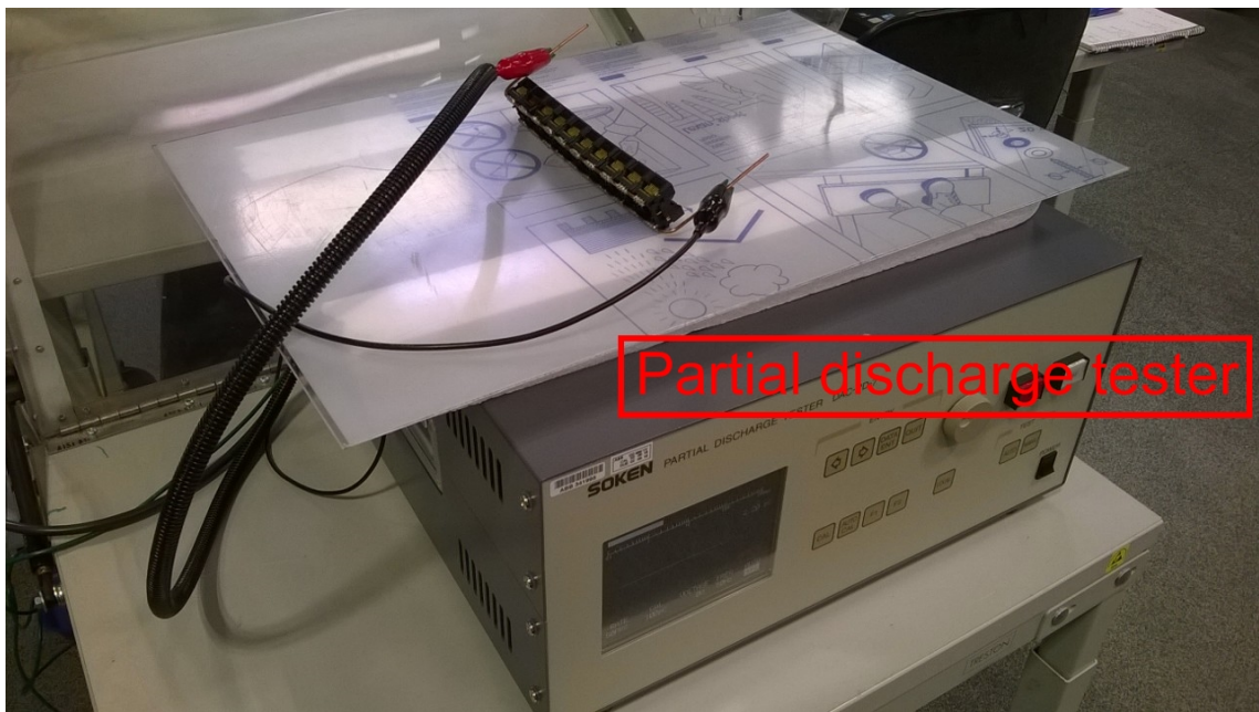
Figure 47: The setup of the partial discharge test.
