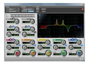
Figure 2: A screenshot of an equalizer curve created with EQ III audio plugin by Avid. A five band equalizer is enough to create complex response curves.
