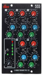
Figure 1: DBX 555 5-band fully parametric equalizer [9]. An example of a five band analog parametric equalizer. Every frequency band is fully parametric and has a control for the gain, the center frequency and the bandwidth. Image adapted from [9].
