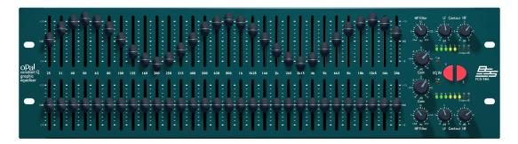
Figure 3: BSS FCS 966 stereo graphic equalizer [10]. An individual equalizer is provided for each of the audio channels. In this design frequency bands range from 25 Hz to 20 kHz with the gain range of  $\pm 15$  dB. The gain faders provide a graphical presentation of the equalization curve. Image adapted from [10].
