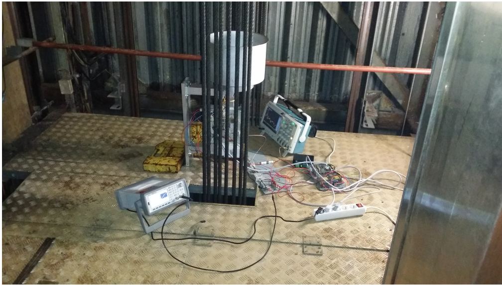
Figure 23: Elva-1 measuring towards the bottom of the elevator car in the elevator shaft of Tytyri.
