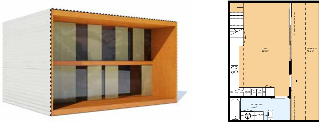
Figure 4.10. An alternative to a transitional shelter: a permanent plywood home for Haiti. © Kombi Architects Ltd.
