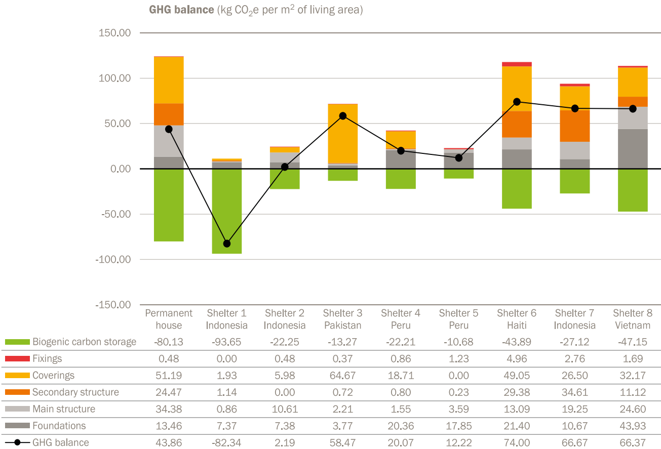
Figure 4.11. A comparison of the GHG balance of a permanent house and eight transitional shelters.
