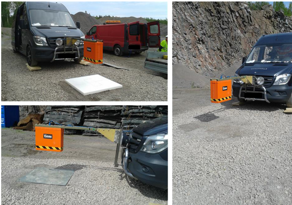
Figure 34: Measurement setup for POM-plate, metal plate on crushed rock, and crushed rock only
