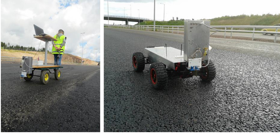
Figure 1: (On the left) Microwave radar installed in a cart, and (on the right) the radio-controlled radar rover
