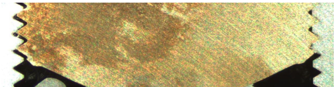
Figure 30 A difference in the shape of the crest is observable when comparing the sides of the internal thread. The crest on the left is sharper. It seems the thread bore and tapping are not entirely concentric.
