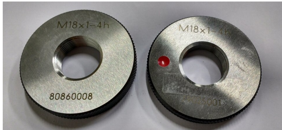
Figure 18 Thread gauges for external M18 x 1 – 4h threads. The rejection gauge marked with a red dot can be seen on the right.
