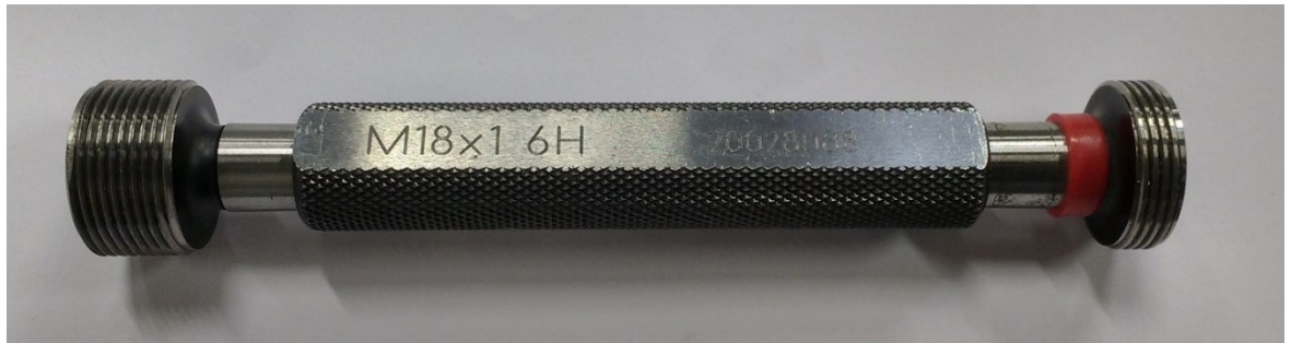
Figure 17 A thread gauge for internal M18 x 1 – 6H threads. The left end is used for verification and the right end marked with red is used for rejecting diverging threads.
