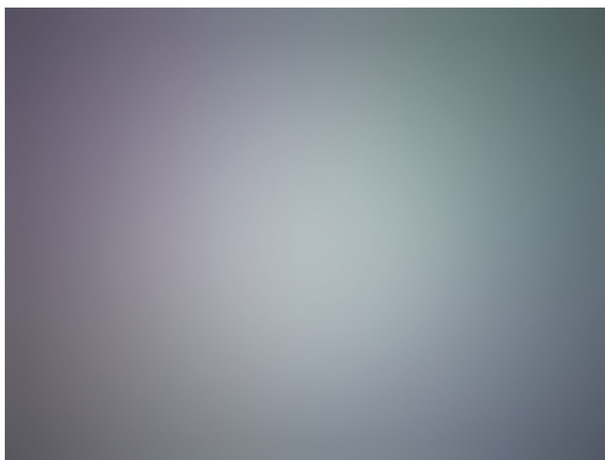
Figure 5.4: Example image of camera color shading. Photograph from I3A CPIQ White Paper. [18]
