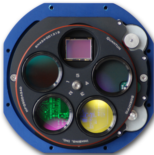
Figure 4.3: A partially disassembled QSI 583 astronomical CCD camera with an integrated filterwheel. Photograph by QSI Press Photos. [11]
