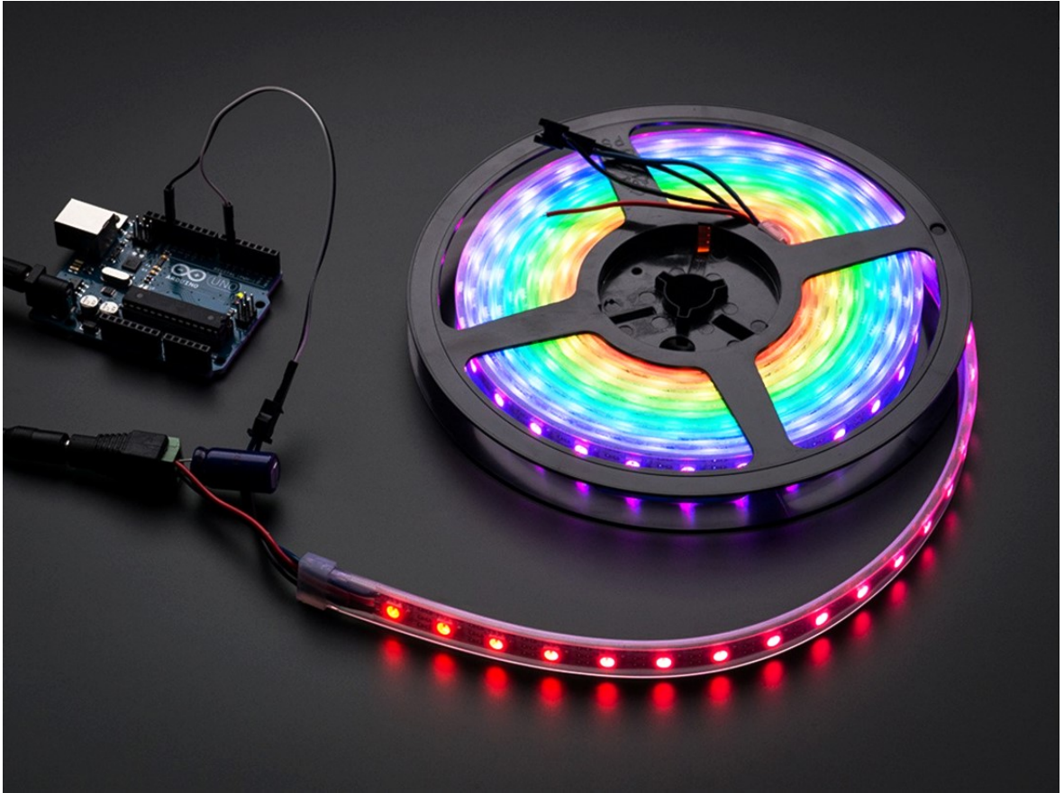
FIGURE 18 ADAFRUIT NEOPixel LED STRIP CONTROLLED WITH ARDUINO UNO, COURTESY OF ADAFRUIT [77]
