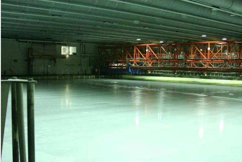
Figure 3.2. Ice tank at Aalto University.
