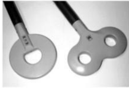
Fig.8 Two types of TMS coil: circular coil on the left and figure eight on the right.
