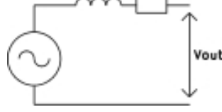
Figure 4: A simple electromechanical generator equivalent circuit. Coil inductance and resistance are modelled as lumped components in series with EMF modelled as voltage source.
