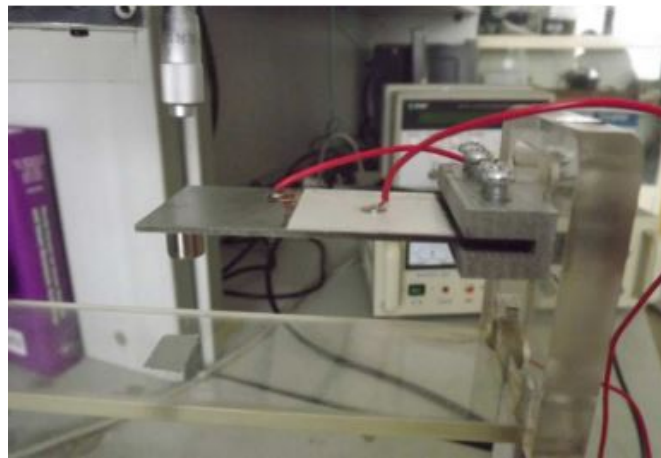
Figure 1: Piezoelectric generator configured as cantilever by Arroyo et al. [13].
